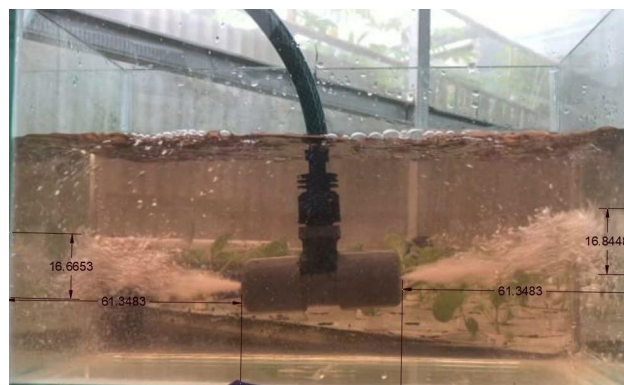
Figure 2. Bubble from the dual nozzle ventury.
